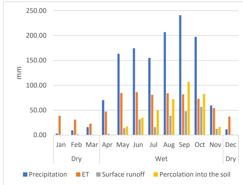
*The components of the water cycle in the Stung Chinit watershed (precipitation, ET, surface runoff and percolation of water into the soil leading to both aquifer recharge and subsurface flow back to the river) by month in millimeters (mm).*
