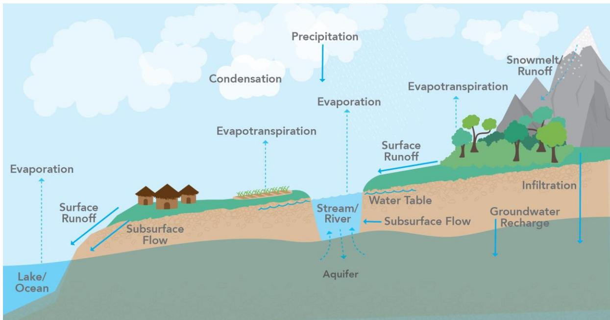
Figure 1. The various movements of water as it moves through the water cycle.
