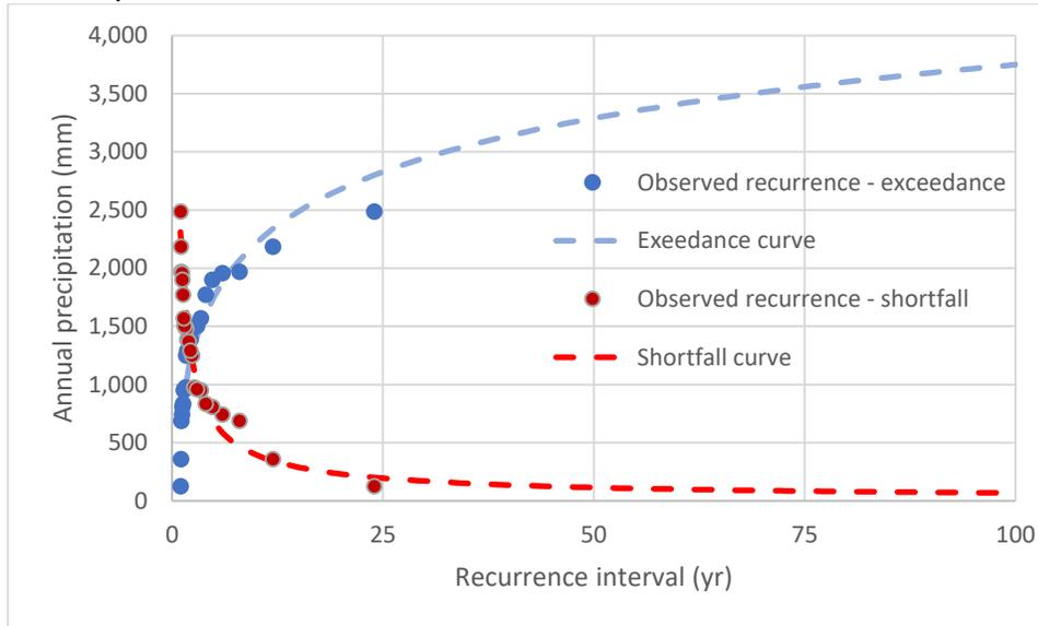
Figure 7. Frequency curve of annual precipitation amounts according to observed rainfall in rain gauges near the Stung Chinit watershed. The exceedance curve shows probability of annual rainfall being **higher** than a given amount, while the shortfall curve shows the probability of annual rainfall being **lower** than a certain amount.
