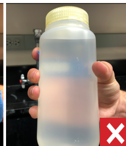
Always use gloves when sampling. If a sample gets contaminated, resample with a backup sample container.
