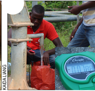
Measure flow rate while sample is collected.
