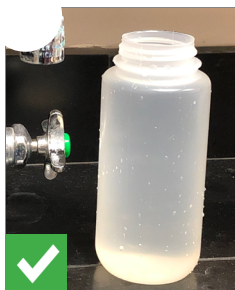
Never touch the inside of the container or the cap to any surface once sterilized. Do not leave samples uncapped.
