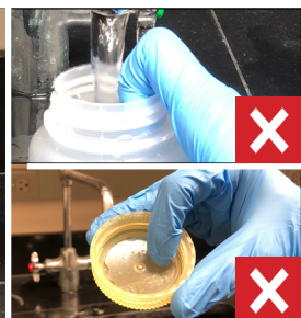
Never touch the inside of the container or the cap to any surface once sterilized. Do not leave samples uncapped.
