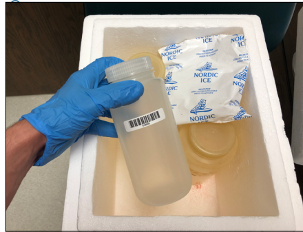
Store samples in a cooler with ice, labeled with barcodes.
