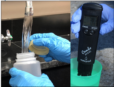
Sample as above and measure for pH and free chlorine residual (FCR) immediately.
