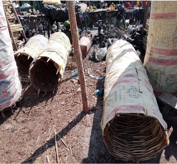
A. Well-built basket rings for toilets at Mandanga Market
