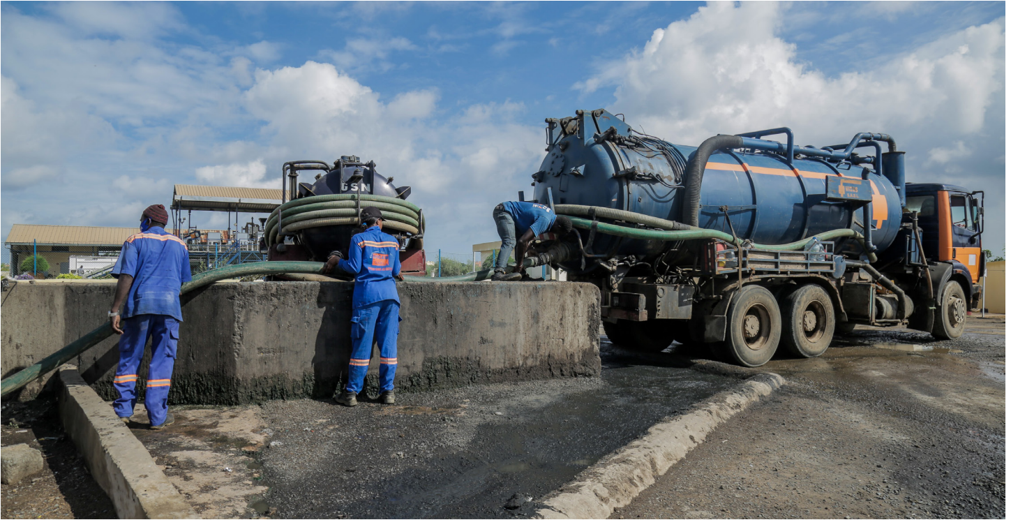
Senegal's only female emptier assists with a fecal sludge emptying operation in a fecal sludge treatment plant (FSTP). Photo credit: WASH-FIN
